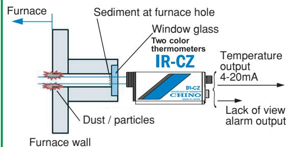
When measuring in a vacuum firing furnace, the field of view may be missing due to dirt on the window glass or deposits on the furnace wall.
